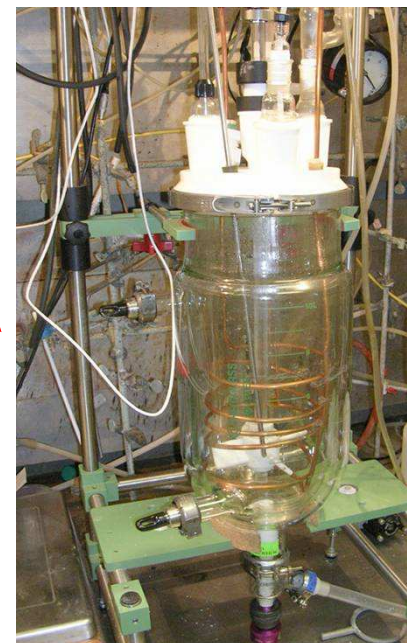
ChemGlass Glass Reactors : 5-100-L scale, unattended dosing and temperature control capabilities
