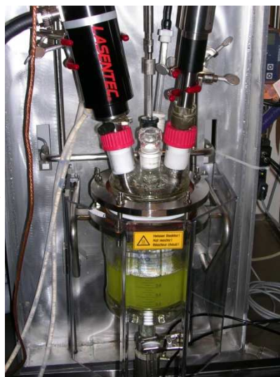
RC1 : 0.08-2-L scale, accurate heat flow on reactions, data collection enhanced with ability to use FBRM, PVM, ReactIR
